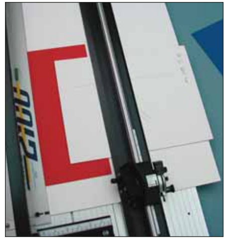
Photo 4: Red mat face-down under the clamp, with drop out underneath aligned to template.
