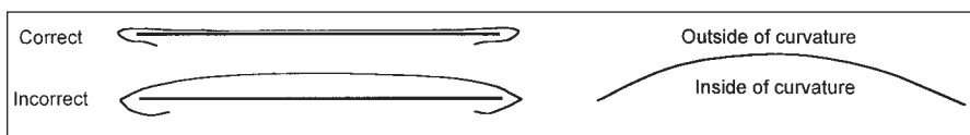
Figure 5: When encapsulating curved objects, it is important to make sure the clear film adheres to the curvature of the item.
