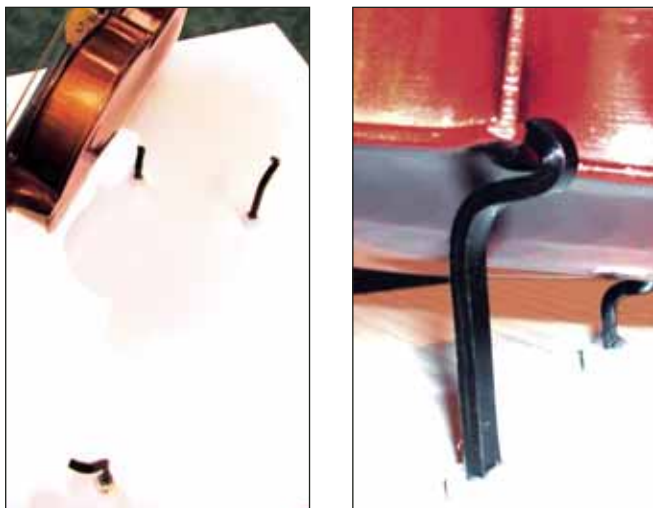
These acrylic mounts have been shaped with heat. A series of acrylic mounts are adhered to a backing board.
