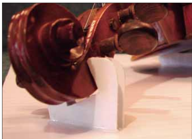
A series of polyflute supports are welded to a backer of the same material. It can be covered with fabric, then the violin placed inside.
