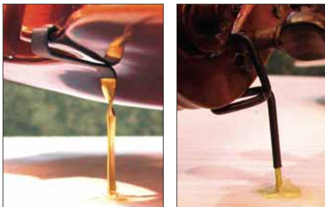
(At left) The brass mounts are inserted, then glued, through the backer. (At right) The tubing over the brass mounts provides a more subtle look.
