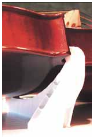
Polyflute is easily cut to form supports of various shapes.
