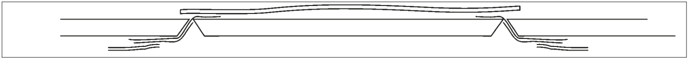
Figure 1: When the hinges are dry and secure, they can be pulled through the slits and secured on the back of the backmat with strips of linen tape.
