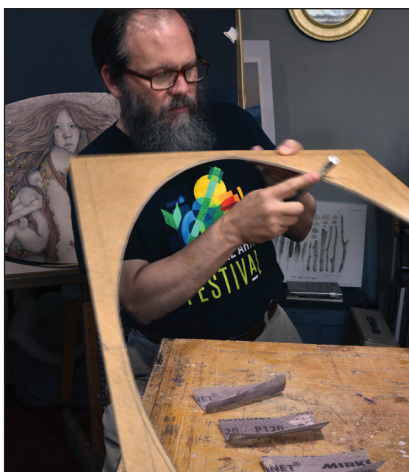
● Shaping the untempered standard spandrel by ensuring the curve never straightens along its continuous path.
