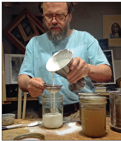
● Straining shop-made gesso made with rabbit skin glue and calcium carbonate (gilder's whiting).
